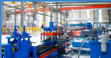
Fully automatic production line for Friction bolt 管缝锚杆全自动生产线
