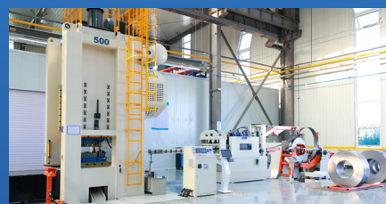
Fully automatic production line for 500t plate 500T托盘全自动生产线
